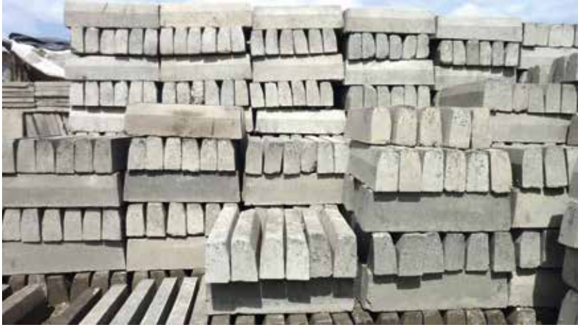
Figure 7: informal street side production of pre-cast concrete parts in Kenya.
