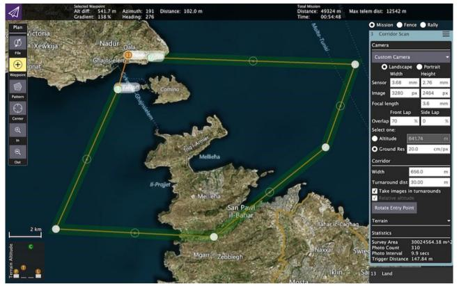
The flightplan is defined before launch on the laptop and then transferred to the drone via the telemetric link. The drone will follow the flight plan fully autonomously. The plane contains a battery that can be charged with supplied charge equipment. The depicted example flight plan with a total flight distance of 50km covers an area of 30 km<sup>2</sup> at at an image ground resolution of 20cm/pixel.
