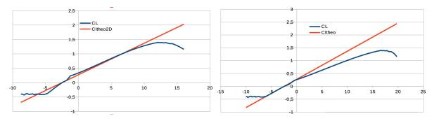
Figure 7: Lift of the infinite wing (left) vs. lift of the finite wing with aspect ration of 5.63 (right)
