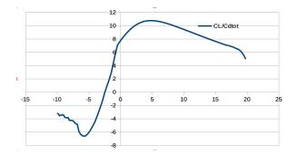
Figure 8:  $C_L/C_D$  vs. angle of attack
