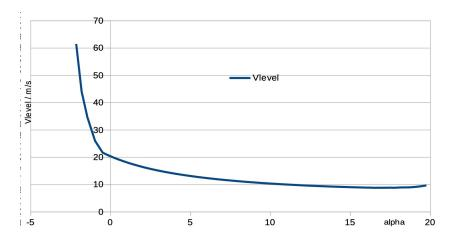
Figure 9: Velocity V for level flight vs. angle of attack
