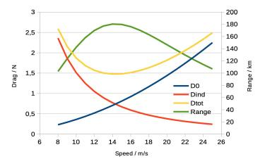
Figure 13: Drag and Range vs. speed for  $C_{D0} = 0.02$
