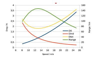
Figure 12: Drag and Range vs. speed
