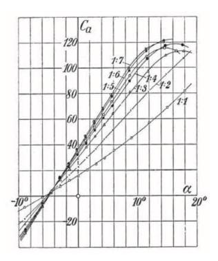
Figure 4:  $C_a$  (=  $C_l$ ) vs. angle of attack for different wing aspect ratios from [3, p.51]
