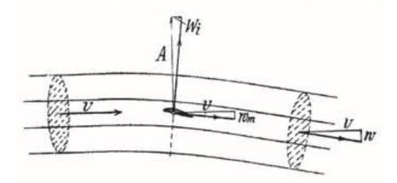
Figure 6: Airflow showing the induced angle  $\alpha_i$  due to induced drag  $W_i$  (from [3][p. 37])
