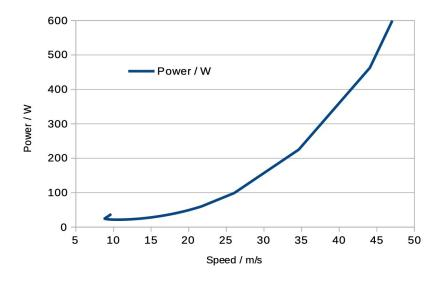
Figure 10: Power vs. speed
