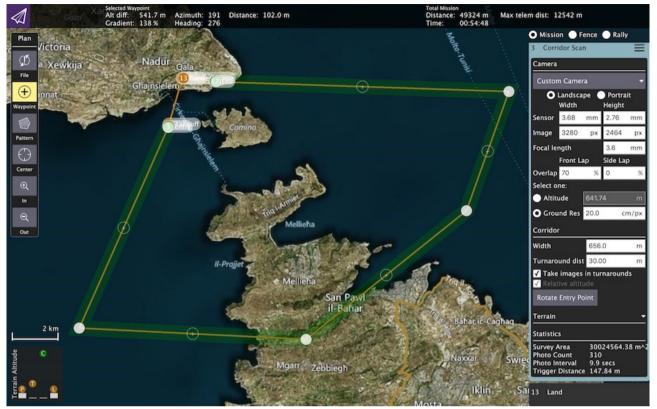
The flightplan is defined before launch on the laptop and then transferred to the drone via the telemetric link. The drone will follow the flight plan fully autonomously. The batteries are charged via the charge equipment. Batteries can be changed, i.e. during flight the next battery can be charged. The depicted example flight plan with a total flight distance of 50km covers an area of 30 km<sup>2</sup> at at an image ground resolution of 20cm/pixel.
