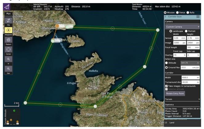
The flightplan is defined before launch on the laptop and then transferred to the drone via the telemetric link. The drone will follow the flight plan fully autonomously. The batteries are charged via the charge equipment. Batteries can be changed, i.e. during flight the next battery can be charged. The depicted example flight plan with a total flight distance of 50km covers an area of 30 km² at at an image ground resolution of 20cm/pixel.
