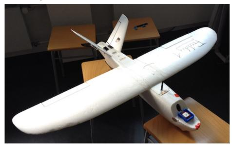
The SearchWing Drone is an autonomous unmanned aerial vehicle that searches for boats on the ocean.
