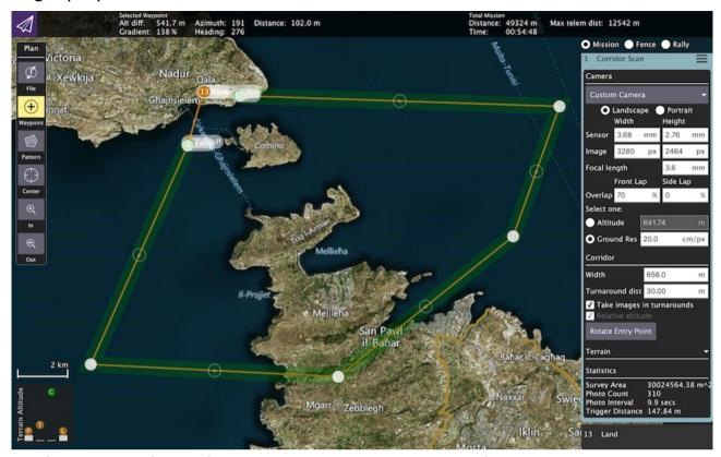
The flightplan is defined before launch on the laptop and then transferred to the drone via the telemetric link. The drone will follow the flight plan fully autonomously. The plane contains a battery that can be charged with supplied charge equipment. The depicted example flight plan with a total flight distance of 50km covers an area of 30 km² at at an image ground resolution of 20cm/pixel.
