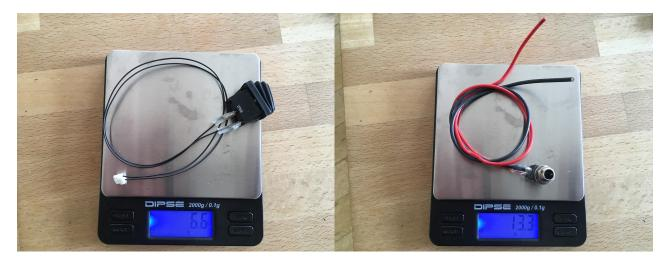
Figure 22: Left: power switch (6.6g), Right: charge connector (13.3g)
