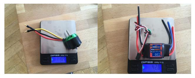
Figure 24: Left: Cobra 2814/20 850kV motor (110.7g), Right: Hobbyking 40A ESC (42.8g)
