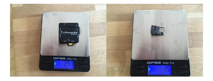
Figure 16: Left: PixRacer with Alu case and memory card (29.1g). Right: Wifi module (1.5g)
