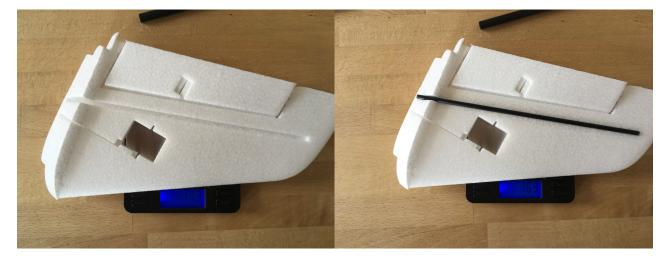
Figure 12: Vtail wing without beam (11.3g) and with beam (16.3g)
