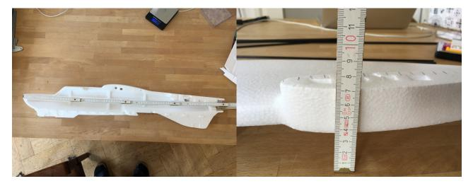
Figure 3: Fuselage length 810mm excluding motor and width 70mm
