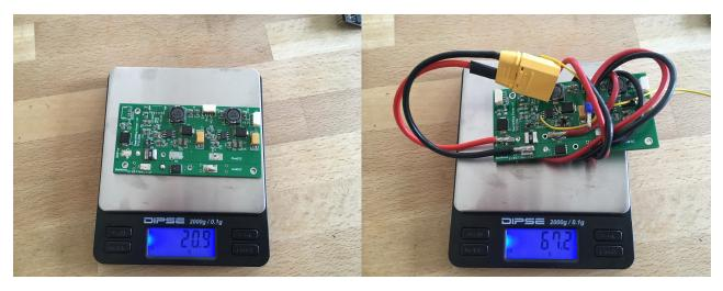
Figure 21: Left: Power module (20.9g), Right: Power module with cable and XT90 (67.2g)
