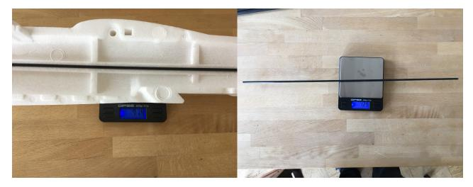
Figure 2: Fuselage half foam and fiber beam 71.4g and fiber beam only with 12.9g
