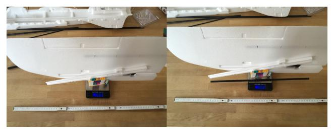
Figure 7: Left wing foam only 107.9g and with fiber beam 120.7g
