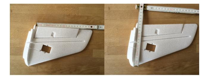
Figure 13: The vtail span is 205mm and has a width of 140mm at the base
