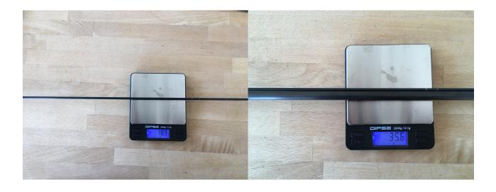
Figure 9: left: wing fuselage rear beam (18.9g), right: wing fuselage rear and front beam (35.6g)
