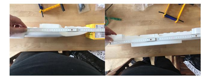
Figure 15: Left: fuselage nose to main wing leading edge 300mm. Right: Main wing leading edge to vtail leading edge 340mm
