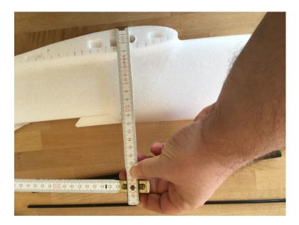
Figure 4: Fuselage height of 120mm
