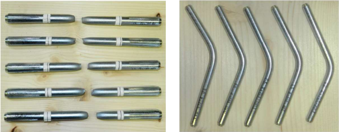
Figure 4.1. 16 mm dowels after tensile tests (left) and 8 mm dowels after bending tests (right)
