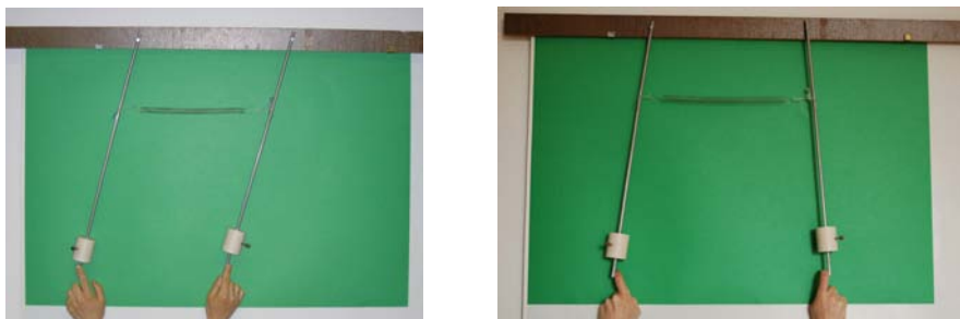
Fig. 2., 3. The two initial conditions which lead to the sinusoidal oscillations.
